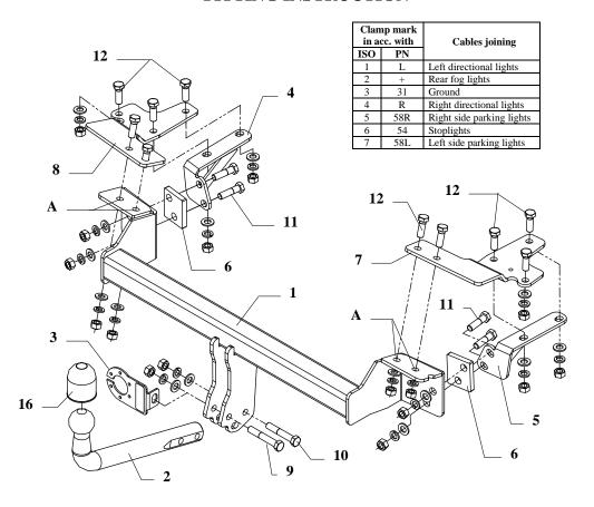
This towbar is designed to assembly in following car: **SUZUKI LIANA, 4 doors,** produced since 03.2002 till 12.2007, catalogue number **W20** and is prepared to tow trailers max total weight **1200 kg** and max vertical load **75 kg**.
